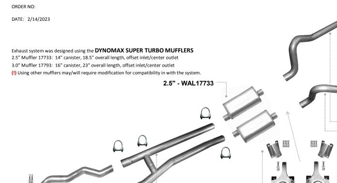
H-PIPE 2-PC ASSEMBLY Includes (5) 3/8" U-bolt clamps.
