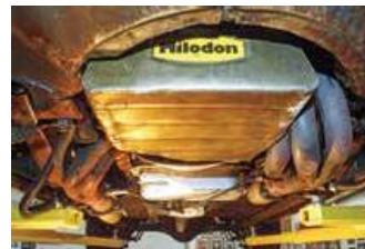
We have had three different pairs of cheap headers on our 340 since 2001. All the headers hung low, which resulted in slightly flattened primary tubes. Each header required one or more tubes to be dinged to fit into the engine bay and around the steering and suspension components. The cheap headers also blew out header gaskets often.
