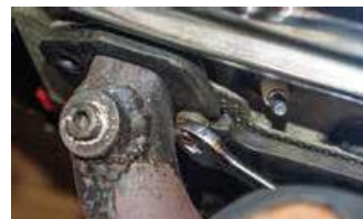
The removal of the header bolts of the old headers was a chore. There was limited clearance between the flange and the primary tube. The header bolts have to be removed a little at a time until the header is free from the cylinder head.
