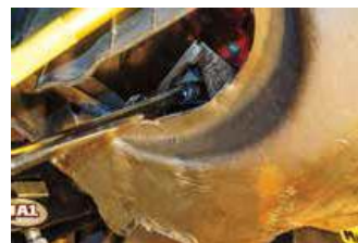
To remove the headers, the engine mount nuts were removed. This would allow us the opportunity to jack the engine up off of the K-member, which would provide additional room to remove the headers.
