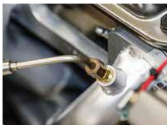
The Percy's EGT probe fit into the header primary tube. The adapter tightened into the bung, and the probe nut secured the probe into the adapter.
