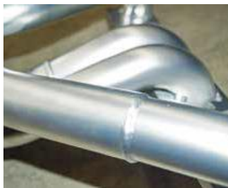
We wanted to see if step headers would improve the performance of our 1969 340 Dart over the cheap, off-the-shelf straight tube headers we have run for years. A presumed benefit of a step header over a straight tube header is they will provide better scavenging, which will broaden the torque curve of the engine.
