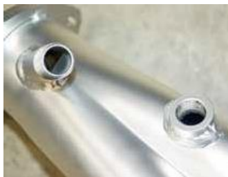
We had TTI install bungs for an oxygen sensor and an evacuation check valve tube into each collector. TTI can install the bungs in the collector or in the reducer/adapters, which is bolted to the collector flange.
