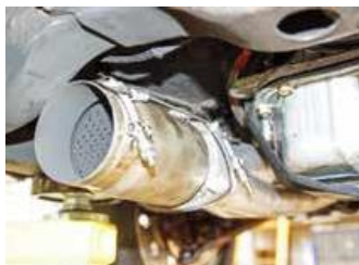
We reinstalled the bullet mufflers onto the TTI headers. The mufflers are much closer to the floorpan and snugly packaged around the transmission. The muffler tethers connected to the TTI header collector properly.
