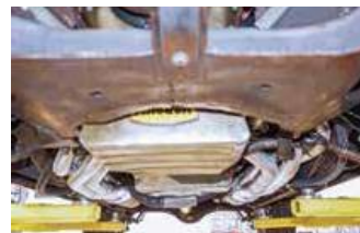
The ground clearance with the TTI headers is greatly improved. TTI packs the pipes much closer to the floorpan and around the transmission. If something hits the ground, it will not be the header pipes.
