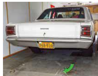
The old headers had been known to hit the floor at the transition from the beaver tail of the trailer to the level floor (green arrow), but with the TTI headers this is a thing of the past. Now if we cannot get the trailer perfectly level or tilted backward slightly, the Dart should still be able to be removed without dragging on the plywood floor.
