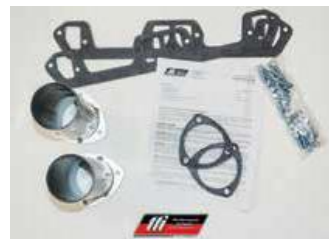
TTI provided an installation kit with the headers. The kit includes gaskets, collector adapters (extensions), all the mounting hardware, and detailed instructions that include installation procedures and maintenance info.
