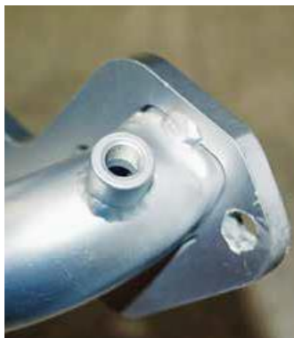
We ordered each header with an exhaust gas temperature (EGT) probe bung welded into the foremost primary pipe (cylinders 1 and 2). TTI took great care to ensure that each bung was placed the same distance from the exhaust valve to provide consistent readings from cylinder to cylinder.
