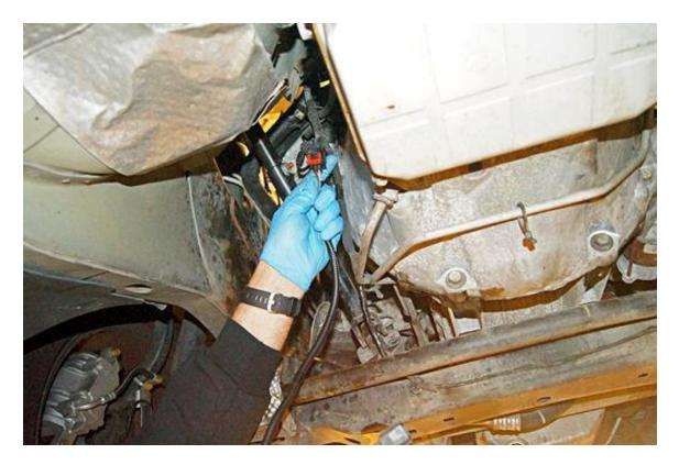
Before the headers were slipped into place, the O2 sensor extension wires were plugged into position. It was easier to install the extensions at this point rather than fight around the headers after the header installation. The extensions were connected and then moved aside to allow the installation of the headers and cats.
