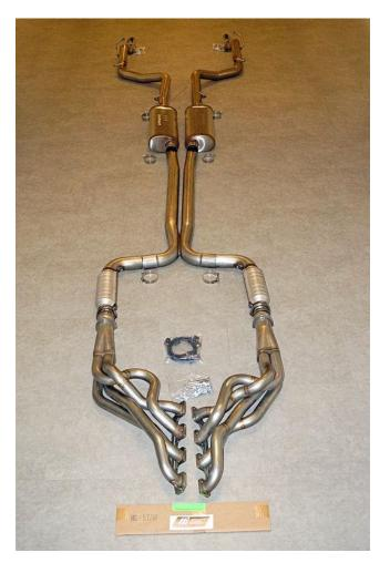
TTi exhaust part no. PK-57XP-MA for the 2005-2015 Chrysler 300, Charger, and Magnum 5.7L Hemis includes a pair of 1 7/8-inch unequal length primary tube headers, two MagnaFlow catalytic converters, a 3-inch x-pipe mid-section, two MagnaFlow mufflers, and a pair of tailpipes with polished 304 stainless tips. Also included is all the necessary mounting hardware, gaskets, O2 sensor extensions, and a dipstick spacer.
