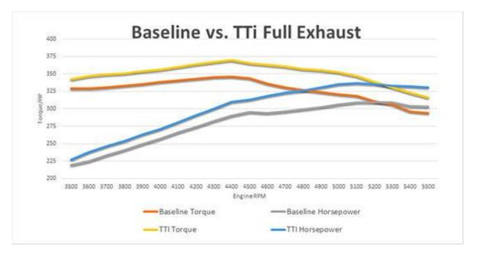
This graph illustrates the baseline torque (orange) and baseline horsepower (gray). The TTi exhaust torque (yellow) jumped up 24 lb-ft to 370 lb-ft at 4,400 rpm, and the TTi exhaust horsepower (blue) was up 28 hp to 337 hp at 5,100 rpm. Undoubtedly, this performance increase can be felt in the seat of the pants and heard by all near the Charger.
