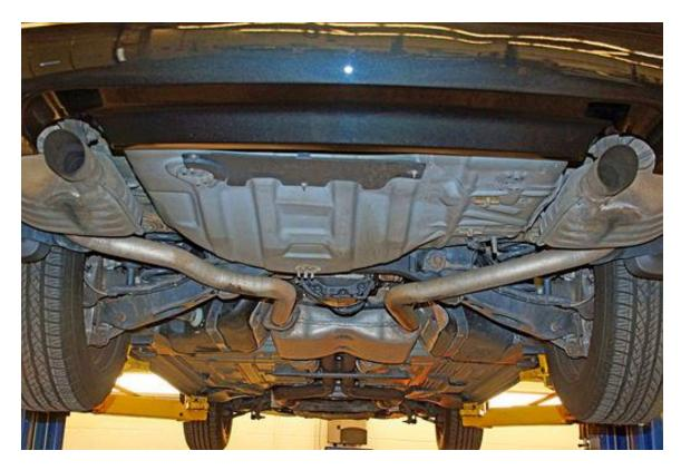
The driver-side tailpipe and muffler assembly was detached from the center muffler. This allowed the tailpipe and muffler to be freed without removing the bumper cover. With the driver-side tailpipe removed, the band clamps were loosened to release the center muffler, mid-pipe, and passenger tailpipe as an assembly.
