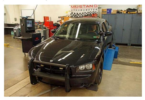
Pennsylvania College of Technology provided their dyno facility for all the testing of the Charger. The Charger with Performance Distributorsø SOS coils, AMSOIL products throughout the drivetrain, and a 93-octane tune laid down a baseline of 346 lb-ft of torque at 4,400 rpm. Baseline horsepower was 309 hp at 5,200 rpm.
