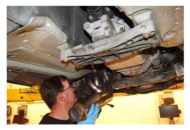
The headers slipped into place with little difficulty. TTi recommends using a thin-layer of high-temp sealer on both sides of the exhaust gasket to ensure a leak-free installation, and the sealer helped to hold the gasket in place during the installation. While many of the header bolts could be accessed from the bottom of the Charger without removing additional components, both motor mounts had to eventually be removed to gain access to some lower and upper header bolts.
