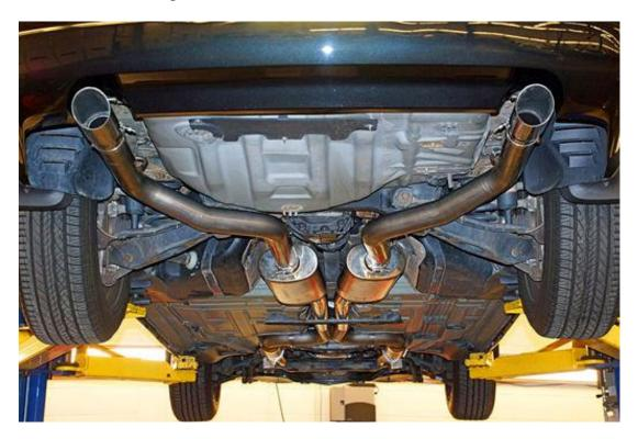
The TTi exhaust used all the factory rubber grommets and factory hangers for the proper fitment. The TTi exhaust flowed from the pair of mufflers to the polished tips that added just a little flash to the exhaust. The tips were fine-tuned for proper fit after the rest of the exhaust had been adjusted. The tips required a small hole to be drilled into the tailpipe and a rivet to be placed into the hole. A band clamp wrapped around the tip, and the rivet held everything in place.
