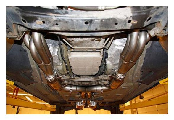
The TTi exhaust fits like a glove. All the factory heat shields were left in their factory location, and the pipes snaked under the chassis in the factory locations without any interference. There was no need for any õhammer modsö to make the exhaust fit into place.
