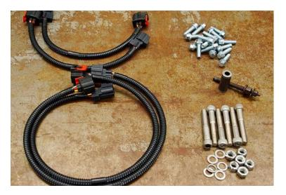
TTi provided all the necessary hardware for the installation of the new exhaust system. Included in the kit are four O2 sensor wiring extensions, 17 header bolts (only 16 bolts may be necessary if one of the factory bolts has to be reused with the provided spacer to locate the dipstick), and six bolts, washers, and nuts for the header collectors.
