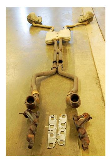
The factory exhaust proved to be functional, but the restrictive exhaust manifolds and multiple mufflers reduced the performance potential of the Hemi. If the exhaust is anything but new, expect to work with plenty of rusted fasteners. Anticipate using plenty of penetrant spray, the use of an array of sockets, ratchets, swivels, extensions, and wrenches to free the exhaust, and, lastly, have plenty of patience while working on this task.
