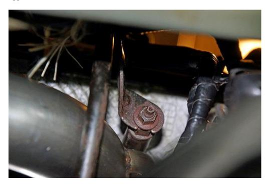
The 5.7L required the use of a factory bolt with the addition of a TTi-provided spacer to locate the dipstick in the proper location. The best factory bolt (not rusted or broken) was selected for this task. The bolt, spacer, and stud did the job, and the dipstick was located in nearly the factory location. The dipstick installation was much easier from under the car rather than attempting to slide the dipstick in to place from the top of the engine bay.
