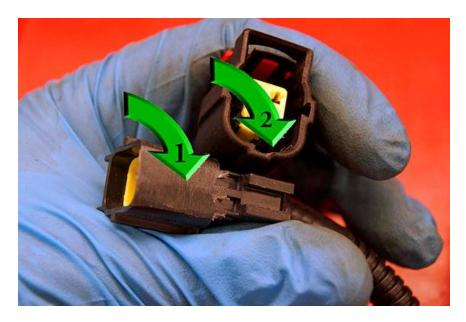
With this Charger, the O2 extension wire connectors had to be modified to fit the factory wiring harness connectors. Arrow õlö shows where a guide rail had to be ground off permitting the male connector to fit into the O2 sensor connector. Arrow õ2ö illustrates the modification to the female connector housing. An offset guide rail was ground into the connector housing to allow the connector to fit into the factory wiring harness. Three of the four connectors required some type of modification.
