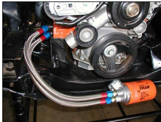
Remote filter mounted for illustration purposes only. Mount your filter to suit your application.
