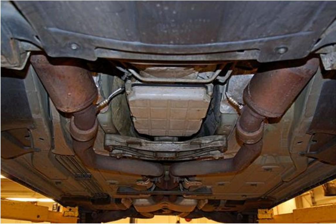
The factory exhaust performed its tasks in decent fashion for the last eleven years. The exhaust consisted of manifolds (not seen), a pair of catalytic converters, an x-pipe converging into a center muffler, and tailpipes that ended in a muffler behind each rear wheel.
