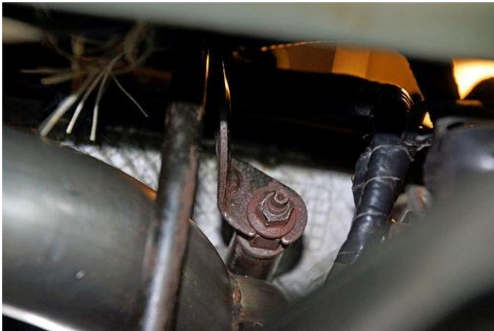
The 5.7L required the use of a factory bolt with the addition of a TTI-provided spacer to locate the dipstick in the proper location. The best factory bolt (not rusted or broken) was selected for this task. The bolt, spacer, and stud did the job, and the dipstick was located in nearly the factory location. The dipstick installation was much easier from under the car rather than attempting to slide the dipstick in to place from the top of the engine bay.
