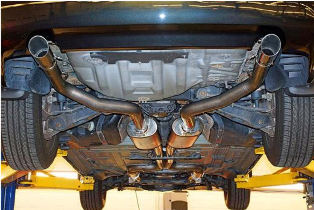
The TTi exhaust used all the factory rubber grommets and factory hangers for the proper fitment. The TTi exhaust flowed from the pair of mufflers to the polished tips that added just a little flash to the exhaust. The tips were fine-tuned for proper fit after the rest of the exhaust had been adjusted. The tips required a small hole to be drilled into the tailpipe and a rivet to be placed into the hole. A band clamp wrapped around the tip, and the rivet held everything in place.
