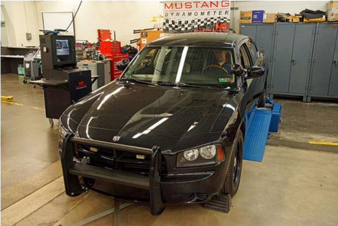
Pennsylvania College of Technology provided their dyno facility for all the testing of the Charger. The Charger with Performance Distributors $\emptyset$  SOS coils, AMSOIL products throughout the drivetrain, and a 93-octane tune laid down a baseline of 346 lb-ft of torque at 4,400 rpm. Baseline horsepower was 309 hp at 5,200 rpm.
