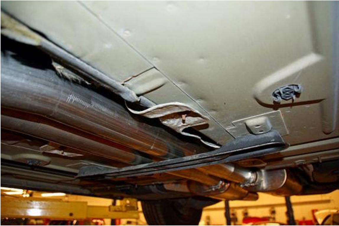
The 3-inch exhaust is very close to making contact with one crossmember located just in front of the mufflers. If necessary, a few washer shims can space the crossmember down a little to increase the clearance of the pipes.
