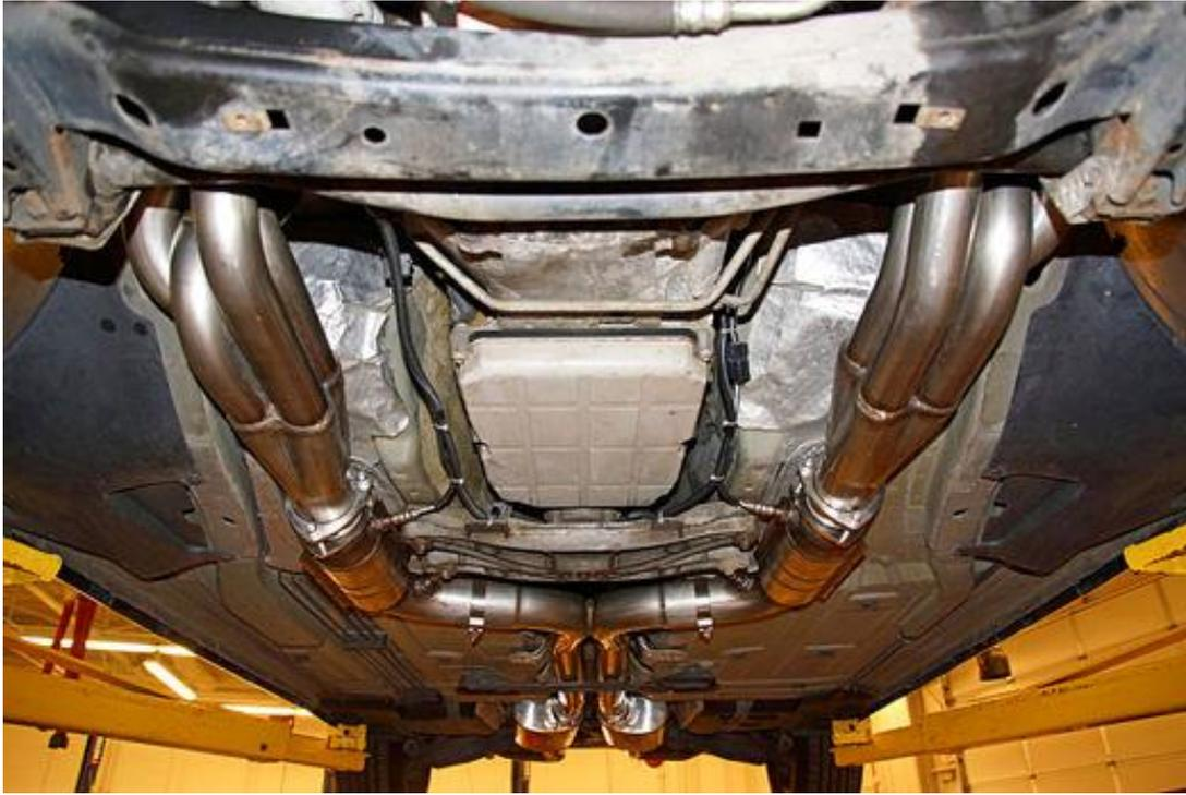
The TTi exhaust fits like a glove. All the factory heat shields were left in their factory location, and the pipes snaked under the chassis in the factory locations without any interference. There was no need for any hammer modsö to make the exhaust fit into place.
