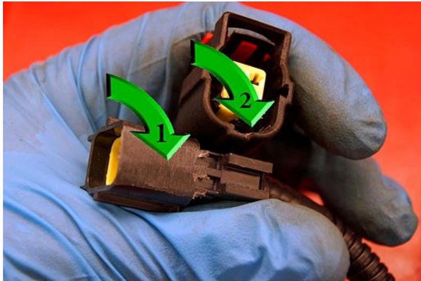
With this Charger, the O2 extension wire connectors had to be modified to fit the factory wiring harness connectors. Arrow "1" shows where a guide rail had to be ground off permitting the male connector to fit into the O2 sensor connector. Arrow "2" illustrates the modification to the female connector housing. An offset guide rail was ground into the connector housing to allow the connector to fit into the factory wiring harness. Three of the four connectors required some type of modification.
