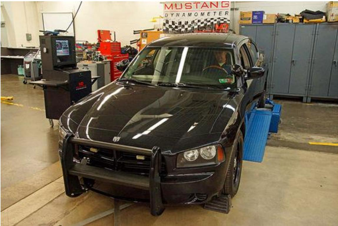
Pennsylvania College of Technology provided their dyno facility for all the testing of the Charger. The Charger with Performance Distributorsø SOS coils, AMSOIL products throughout the drivetrain, and a 93-octane tune laid down a baseline of 346 lb-ft of torque at 4,400 rpm. Baseline horsepower was 309 hp at 5,200 rpm.
