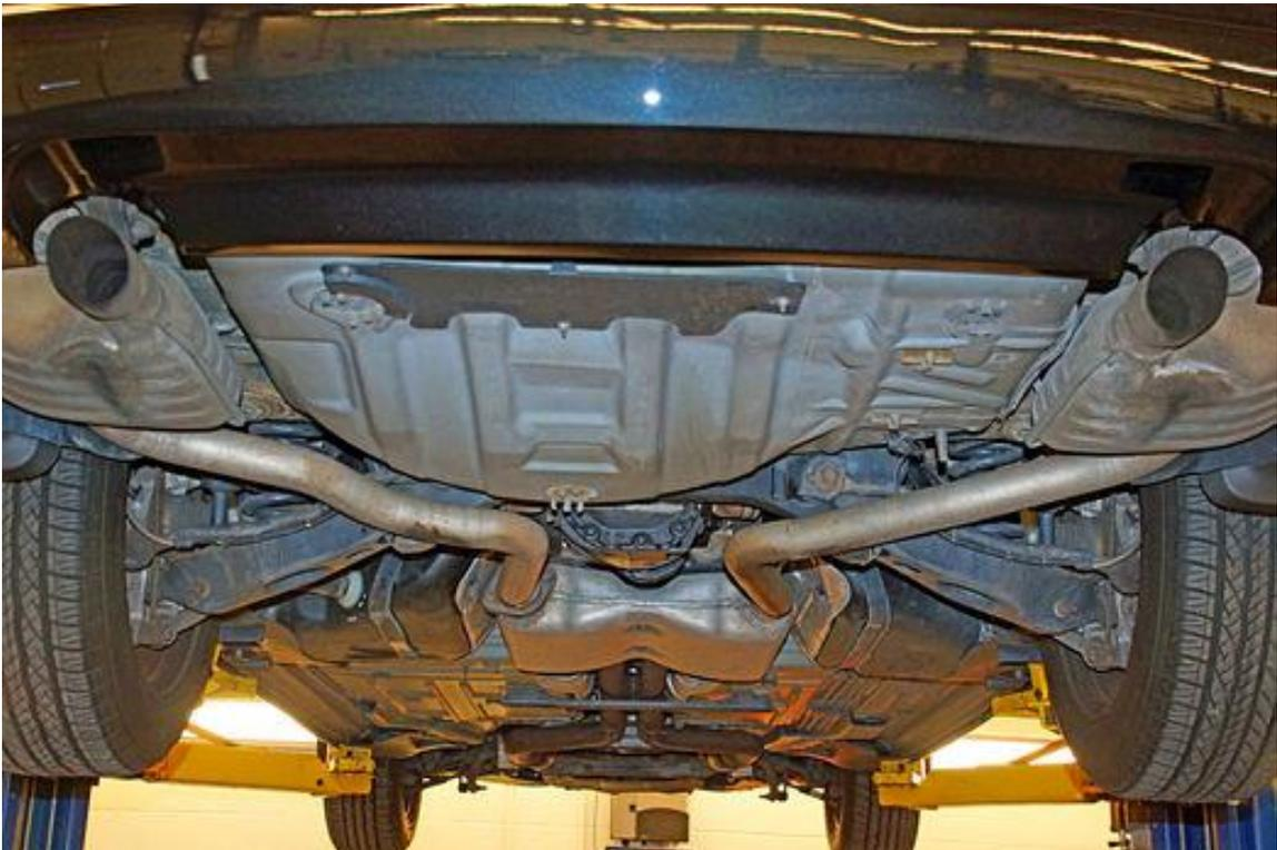
The driver-side tailpipe and muffler assembly was detached from the center muffler. This allowed the tailpipe and muffler to be freed without removing the bumper cover. With the driver-side tailpipe removed, the band clamps were loosened to release the center muffler, mid-pipe, and passenger tailpipe as an assembly.
