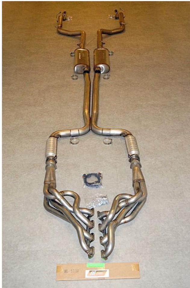
TTi exhaust part no. PK-57XP-MA for the 2005-2015 Chrysler 300, Charger, and Magnum 5.7L Hemis includes a pair of 1 7/8-inch unequal length primary tube headers, two MagnaFlow catalytic converters, a 3-inch x-pipe mid-section, two MagnaFlow mufflers, and a pair of tailpipes with polished 304 stainless tips. Also included is all the necessary mounting hardware, gaskets, O2 sensor extensions, and a dipstick spacer.
