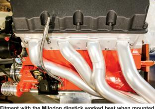
Fitment with the Milodon dipstick worked best when mounted and routed as seen here. Routing/mounting it any differently made pulling and putting in the dipstick very difficult, if not impossible.
