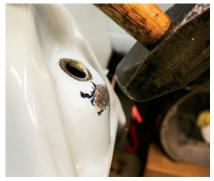
We tried an air hammer, but our trusty old 3-pound mini sledgehammer did the job. It took a few hundred blows of our hammer to reshape the 1/8-inch-thick metal and bend it back about a half-inch. Fact: The early B-Body shock tower bulges out further than the '66-and-later B- and E-Body shock tower, plus the engine sits a ½-inch further to the right.
