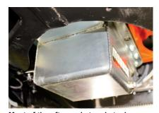
Most of the aftermarket and stock Hemi/wedge oil pans are designed for fitment with the '66 and later B- and E-Body. Using the aforementioned oil pans require the early B-Body K-member to be notched. Not so with this deep 7-quart Moroso oil pan (PN MOR-20760, Summit, \$199.99). This stronger-than-stock oil pan provides plenty of K-member clearance in an early '62-'65 B-Body with a wedge or Hemi engine installation.
