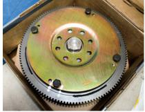
Before installing a transmission, torque converter, and flexplate into a car, it's easier to line up the bolt pattern. Notice the white paint lines on the converter and flexplate. The 10-inch TCI Ultimate Street Fighter torque converter and the solid TCI eight-bolt Hemi flexplate will handle over 1,000 hp. Both were previously featured in our "Tough Torque Converter" story.
