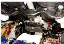
To be sure of proper engine position, we bolted up our A&A trans with the Schumacher mount and stock crossmember. Now we could be exactly sure of where the valve cover was hitting the shock tower. At this point all other clearance checks looked good and the car's original '65 cable-shift, slipyoke Torque-Flite was back in its original location.
