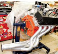
We're glad we straightened out the aforementioned clearance issues before implanting the Hemi into the engine bay. It would've been much more difficult and time consuming to work out the fitment of the headers to starter, block, engine mount, and dipstick inside the engine compartment.
