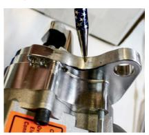
Wanting to keep flying metal chips away from our expensive Hemi, so outside our garage with a die grinder, we shaved an 1/8-inch from the starter's mounting block. No fear, the mounting block of this powerful starter is made of strong billet aluminum versus the cast aluminum of cheaper units.
