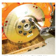
ARP crankshaft bolts (PN ARP-200-2905, Summit, \$33.95) were used to secure the TCI solid flexplate. The ARP fasteners received three steps of torque (40 to 60 to 85 ft-lb) in a crisscross torque sequence pattern.
