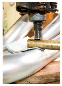
The headers easily bolted in without the torsion bars in place. Only the left side requires the engine to be raised an inch. Once installed, the L/S side header touched the Borgeson quickratio power steering box. The R/S header was rubbing the torsion bar. Shown here, we're dimpling the R/S header using a hydraulic press, piece of leather, 1-inch brass drift and a few blocks of wood while trying not to scratch the ceramic coating on the TTI headers.
