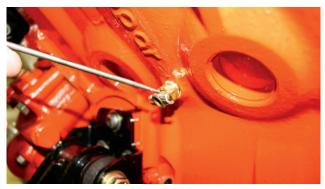
With our Hemi on the engine stand, it's also much easier to check clearance between the headers to starter, dipstick, engine mounts and block. We discovered trying to bolt on the left-side headers that the radiator petcock was interfering with header fitment. A stock coolant plug was put back into the block for our first clearance correction.
