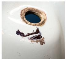
The scratched paint reveals where the valve cover was rubbing up against the shock tower. We used black magic marker to mark the area we needed to beat back the shock tower about a half-inch for the larger Barton valve cover to clear. If our '65 was equipped with an A-990 shock tower, the taller and wider Barton valve cover would have plenty of clearance.
