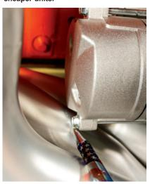
Now, with the starter being able to be bolted up in position, the headers were hitting the starter where the pen is pointing. To remedy this clearance issue, we only needed to clock the starter clockwise one position out of the four available on this clock-able starter.
