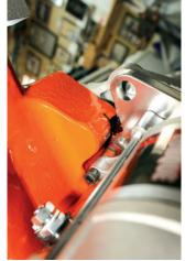
The newer Mopar Gen II Hemi blocks are beefier than the original factory castings. To line up the starter boltholes, we'd need to clearance grind the block or starter. TTI Exhaust recommends use of this clock-able Powermaster XS Torque starter (PN PWM-9523, Summit, \$308.99) for fitment with their headers.
