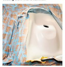
After clearance messaging the shock tower back by over a half inch, that area was sanded smooth and coated with Eastwood gray epoxy primer (PN 14149Z, Eastwood, \$22.99) for good rust protection. Online we found a spray can of B1 Blue to spot-in our handiwork. It's a shade darker than the powder blue, but most folks won't notice.
