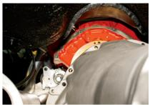
To make life easier, and this is for all classic Mopar V-8s with headers, put the starter in its place resting on the header tubes (as seen) before bolting the transmission or bellhousing to the block.
