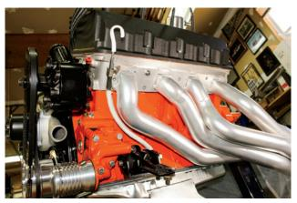
We found the reproduction Street Hemi dipstick fits nicely. It only required minor bending to provide good clearance away from the ceramic-coated TTI 2 1/4-inch headers (PN HEMI625-214C4, TTI, \$977) and Schumacher Creative Services conversion Hemi engine mounts (PN B625H, Schumacher, \$259).
