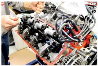
We decided it would be easier to check and set the valve lash on our Street Hemi before dropping it into the tight-fit engine bay. Hemi valve covers — especially our taller and wider Ray Barton units, are easier to remove and reinstall while on the engine stand. Check out the Ray Barton rocker system. It has valvetrain stability up to 10,000 rpm.
