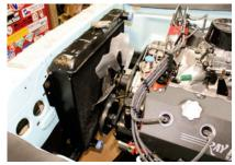
For our final clearance check we hoped an original, air conditioning, aluminum-bladed clutch fan setup ('64-'65 wedge) would fit with the thicker-than-stock, four-row U.S. Radiator. Fortunately, it fit with 5/8- to 11/16-inch clearance, but the 54-year-old clutch unit has shaft wobble. We didn't want to purchase an expensive repo fan clutch for over \$200.
