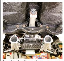
Surprisingly, all-around clearances are better with the TTI 2½-inch Hemi than the TTI 2-inch headers in my 440-powered '67 Coronet R/T. Access to wrench bolts and install accessories are better too. We coated the trans crossmember with Eastwood's 2K Ceramic Aerosol Chassis Black (PN 14146Z, Eastwood, \$24.99) and the undercarriage with Chassis Black (PN 10043ZP, Eastwood, \$34.99 quart) for a clean, cool look.
