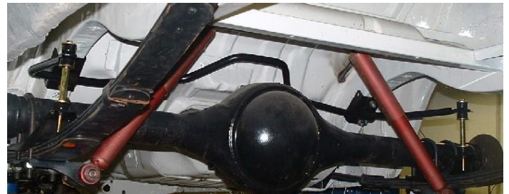
Tailpipes will not clear the FFI sway bar. [Firm Feel, Inc. rear suspension]
