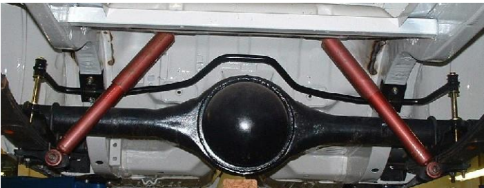
Tailpipes will not clear the FFI sway bar. [Firm Feel, Inc. rear suspension]
